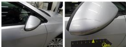
Door R L, Bad repair, LI - Repair and paint (complete)
