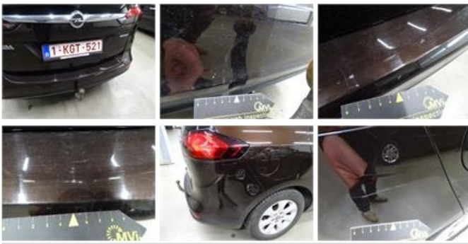
Wing R R, Scratch(es), LI - Repair and paint (complete) 0,00
