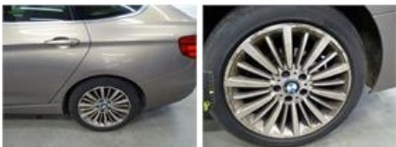
Tyre R R, Deformed / Strained, E - Replace
