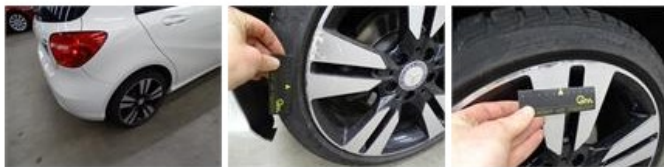
Alloy rim R R polished, Scratch(es), LI - Repair and paint (complete)
