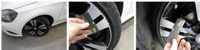
Alloy rim R R polished, Scratch(es), LI - Repair and paint (complete)
