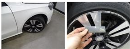
Alloy rim R L polished, Scratch(es), LI - Repair and paint (complete)
