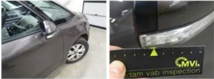
Mirror side blinker R, Crack, E - Replace
