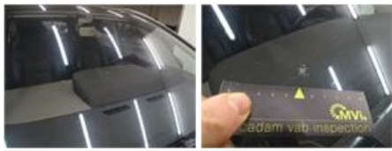
Roof, Dent(s), PDR - Paintless dent repair
