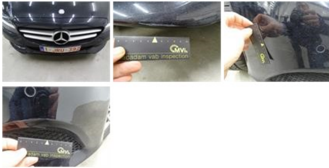
Rocker panel inner F R, Dent(s), LI - Repair and paint (complete)
