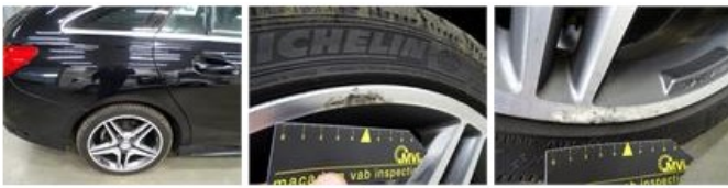
Alloy rim F R polished, Scratch(es), LI - Repair and paint (complete)
