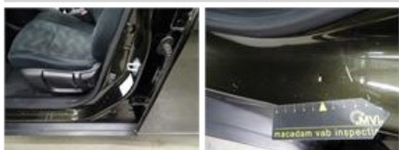
Rocker panel inner R R, Scratch(es), Forfeit
