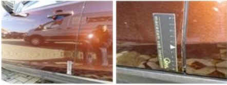
Door R R, Scratch(es), It - Spot repair
