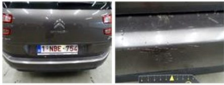
Sill outer R, Dent(s), Le - Replace and paint
