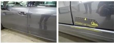
Sill outer R, Scratch(es), It - Spot repair
