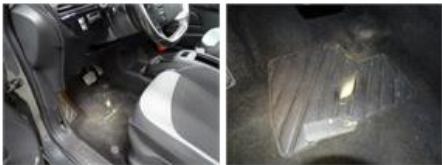
Floor covering F L, Tear, E - Replace
