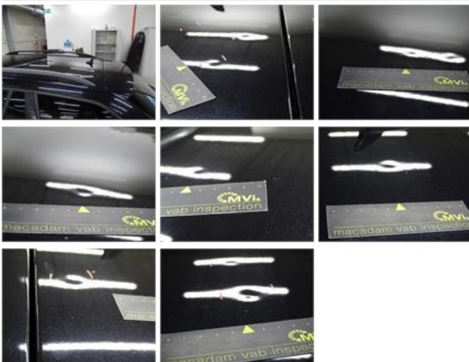
Bumper F, Scratch(es), LI - Repair and paint (complete)
