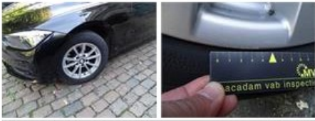
Wing F L, Dent(s) and scratch(es), LI - Repair and paint (complete)
