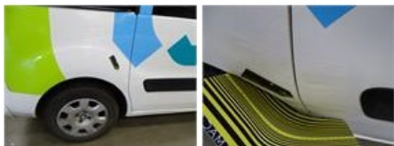
Door R R, Dent(s), LI - Repair and paint (complete)
