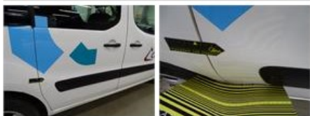
Sill outer L, Scratch(es), It - Spot repair
