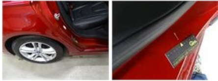
Sill outer R, Scratch(es), LI - Repair and paint (complete)
