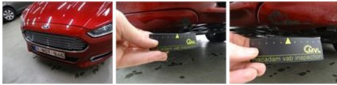
Rocker panel inner R R, Dent(s), LI - Repair and paint (complete)
