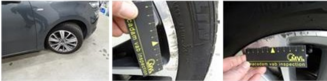
Alloy rim R L polished, Rust, Acceptable
