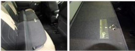
Protection plate M, Deformed / Strained, E - Replace
