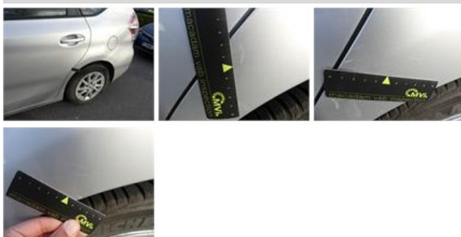
Door frame R R, Dent(s), It - Spot repair
