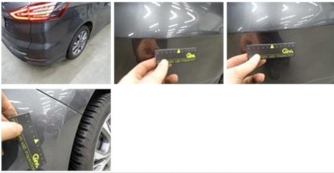
Bumper F, Scratch(es), LI - Repair and paint (complete) 254,16
