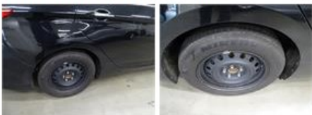
Wheel cover R L, Missing, E - Replace
