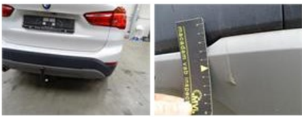
Bumper moulding R R, Deformed / Strained, E - Replace
