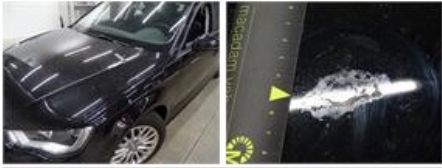
Bumper F, Broken, Le - Replace and paint
