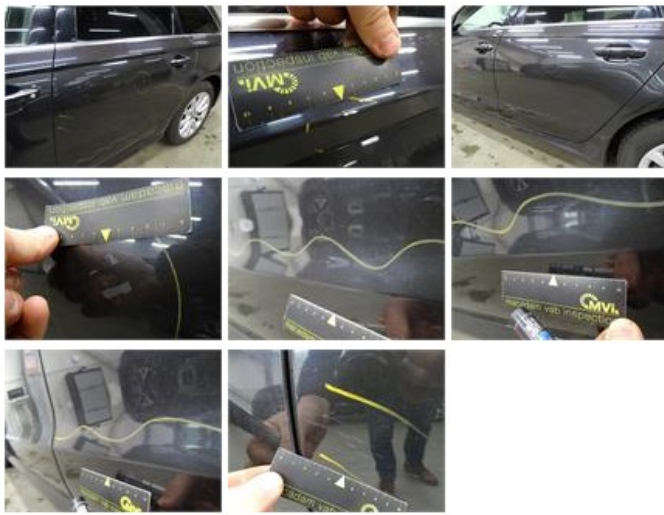
Door F L, Scratch(es), LI - Repair and paint (complete)
