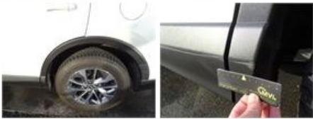
Door R L, Dent(s), LI - Repair and paint (complete)
