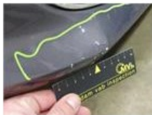
Seat cover R R, Deformed / Strained, P - Check
