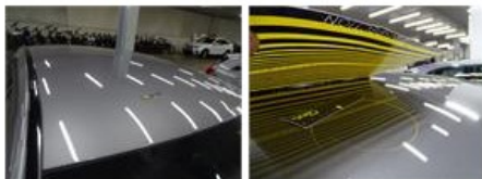
Wing F L, Deformed / Strained, LI - Repair and paint (complete)
