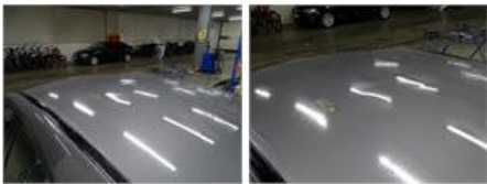
Roof, Deformed / Strained, LI - Repair and paint (complete)
