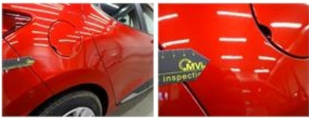
Wheel cover F R, Scratch(es), E - Replace
