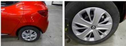
Wheel cover R R, Scratch(es), E - Replace
