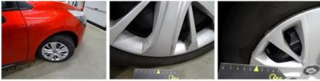
Wheel cover F L, Scratch(es), E - Replace
