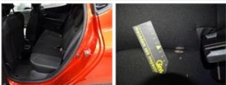
Seat cover R, Burned, E - Replace
