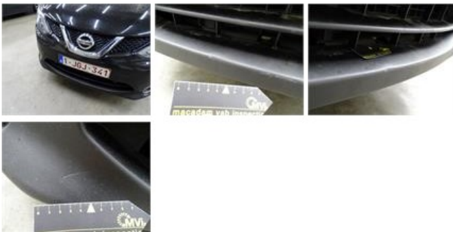
Engine protective plate, Deformed / Strained, E - Replace
