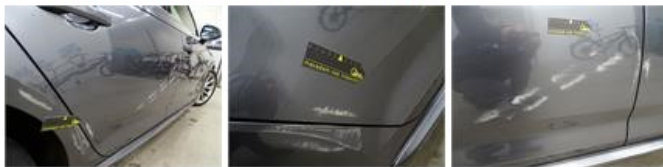
Outer door handle F R, Scratch(es), LI - Repair and paint (complete)
