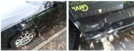
Bumper moulding F R, Missing, E - Replace
