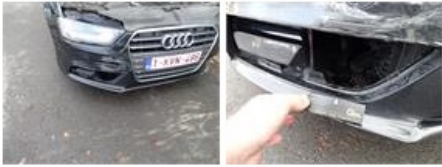
Bonnet, Deformed / Strained, Le - Replace and paint
