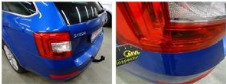
Rearlight L, Crack, E - Replace
