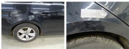
Wing R L, Bad repair, LI - Repair and paint (complete)
