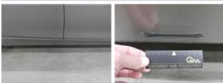
Sill outer L, Scratch(es), It - Spot repair
