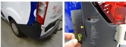
Wheel cover R R, Broken, E - Replace
