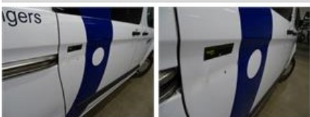
Wing R L, Deformed / Strained, Le - Replace and paint
