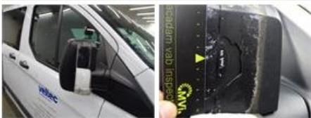
Door R R, Deformed / Strained, LI - Repair and paint (complete)
