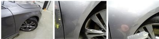
Alloy rim F R, Scratch(es), LI - Repair and paint (complete)
