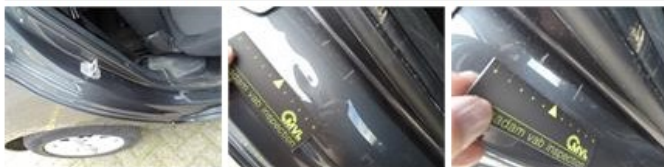
Inner door sill RL, Dent(s), LI - Repair and paint (complete)
