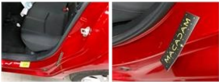
Door FL, Scratch(es), Repair and paint (complete)
