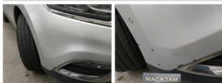
Bumper moulding R, Scratch(es), Spot repair
