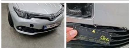
Bumper F, Broken, Replace and paint
