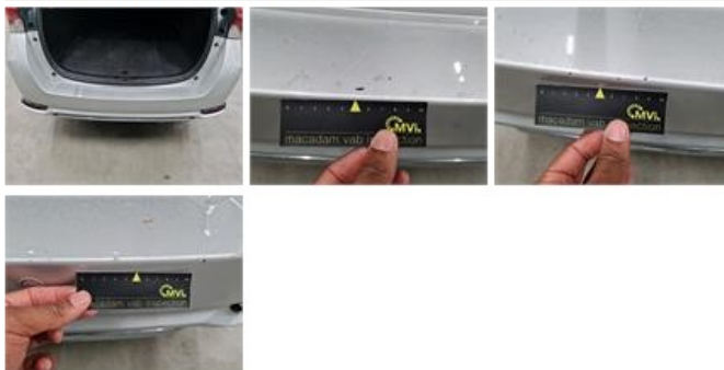
Bumper moulding F, Broken, Replace
