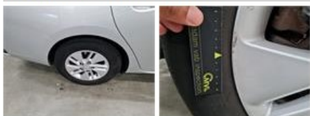
Wing FL, Dent(s), Paintless dent repair
