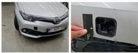
Boot lid covering R, Scratch(es), Smart repair
