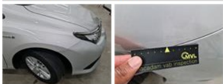
Bumper F, Broken, Replace and paint
