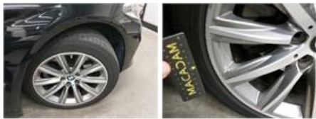
Alloy rim RR polished, Scratch(es), Repair and paint (complete)
