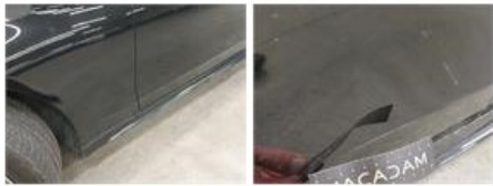
Wing RL, Chemical polution, Repair and paint (complete)
