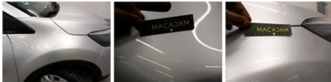
Tailgate / Boot, Bad repair, Check
