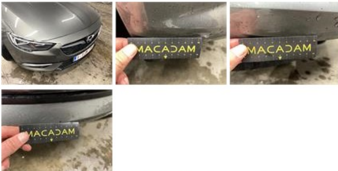
Outer sill L, Dent(s) and scratch(es), Repair and paint (complete)
