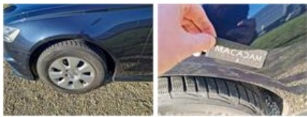
Sill trim R, Scratch(es), Acceptable
