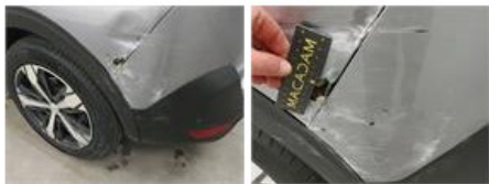
Wing RL, Deformed / Strained, Replace and paint
