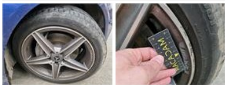
Alloy rim FL polished, Scratch(es), Acceptable
