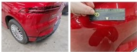
Door RR, Scratch(es), Repair and paint (complete)
