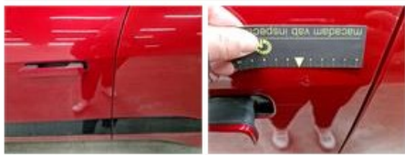
Door RL, Scratch(es), Repair and paint (complete)
