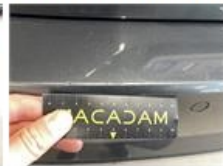
Bumper R, Scratch(es), Repair and paint (complete)
