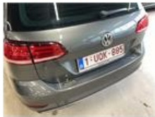
Bumper R, Scratch(es), Repair and paint (complete)
