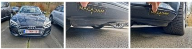
Alloy rim RR, Scratch(es), Repair and paint (complete)
