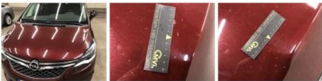
Wing RR, Dent(s), Replace and paint
